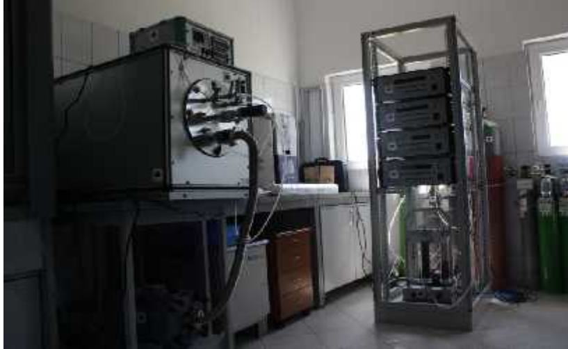
Fig.3. Reference analyzers for SO 2 , CO, NO x (NO, NO 2 ) and O 3
