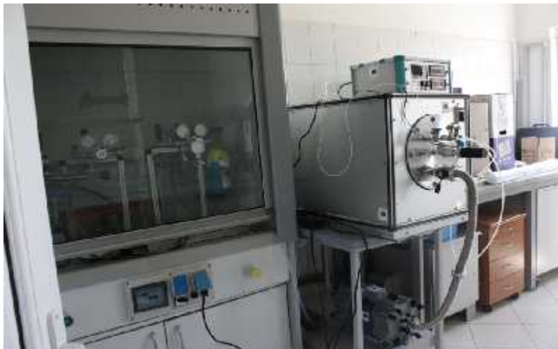
Fig.2. Volumetric system to produce standard gas
