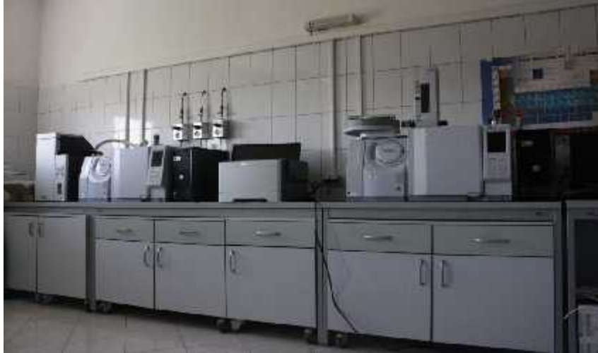
Fig.7. Equipments for organic compounds determinations- GC-MS and GC-MS with TD
